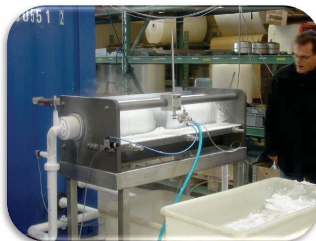
Shock freezing of cellulose fibers. -80^{\circ}\text{C} plant
