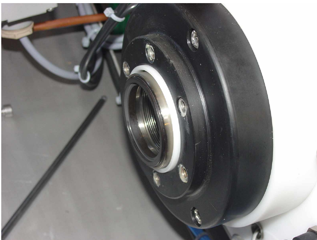
Picture 16 - mount the stop ring
