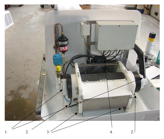
Release the pressure of the machine by running pump down. If any pressure of refrigerant is present you must take off this before opening.
